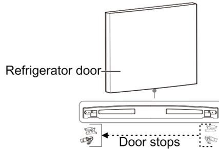
11. Install the refrigerator compartment door.
