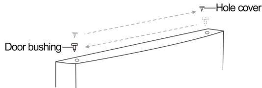
18. Remove the hole cover from the top left side of the cabinet and secures the cover on the top right side of the cabinet.
