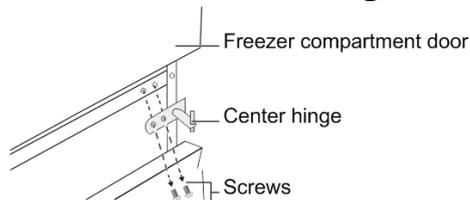
5. Remove the refrigerator compartment door.
