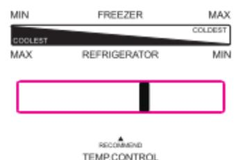
2. When the temperature mode keeps unchanged, adjust the air regulating rod from right to left, the fridge temperature gets decreased while the freezer temperature increased .
