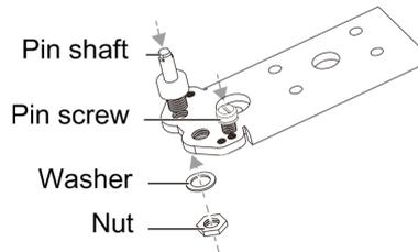
9. Install the lower hinge on the left side of the cabinet.
