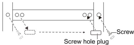
14. Install the center hinge to the left side with the two screws you removed previously.
