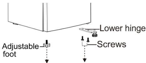
5. Remove the adjustable foot on the lower hinge shaft, and remove the washer and nut.
