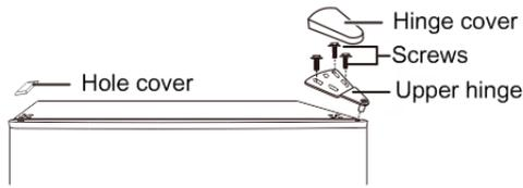
3. Remove the refrigerator compartment door from the cabinet.
