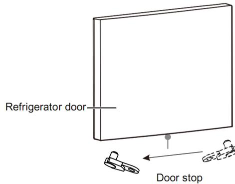
10. Install the refrigerator compartment door.
