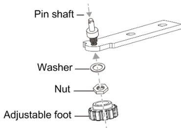
8. Install the lower hinge on the left side of the cabinet. Install the adjustable foot at the right.
